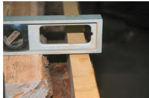
Figure 6 While leveling the board, do not raise the level.
