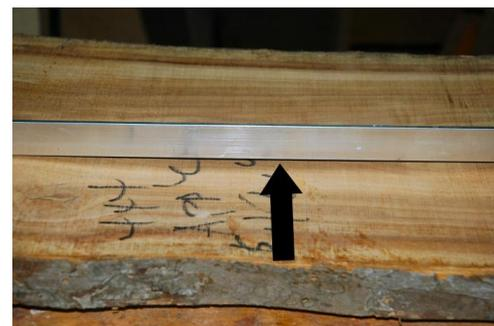
**Figure 10** Find the lowest spot on the board
