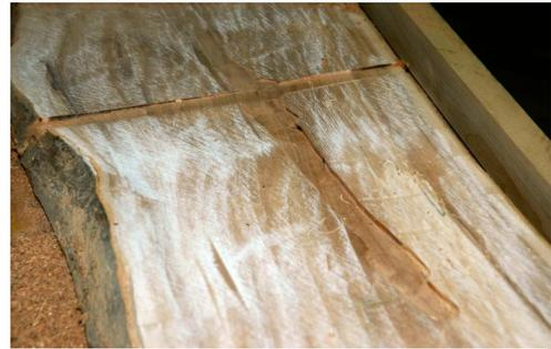
Figure 12 Cut segment lines to make sure that the router bit has not slipped
