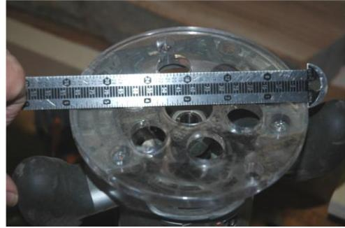
**Figure 7** Measure the diameter of the router base. This measurement will be used a couple of times
