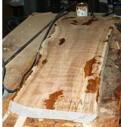
Figure 14 Fill in any cracks, splits, holes and then sand again
