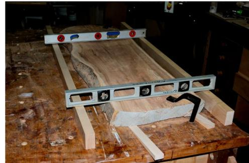
Figure 5 Place 2 straight edges across the rails
