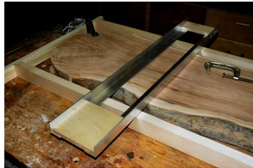
**Figure 8** Place cut boards at each end of the rails
