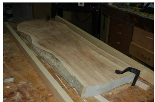
Figure 4 Cut base rails and place parallel near board
